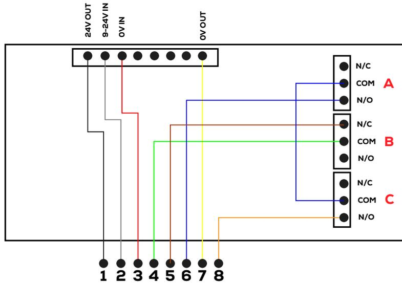
**FILTER CONIDITION ALARM** (Changeable between N/O and N/C in the setup menu)
