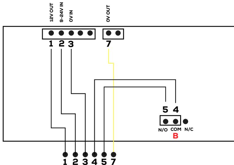
**FILTER CONDITION ALARM** (Changeable between N/O and N/C in the setup menu)
