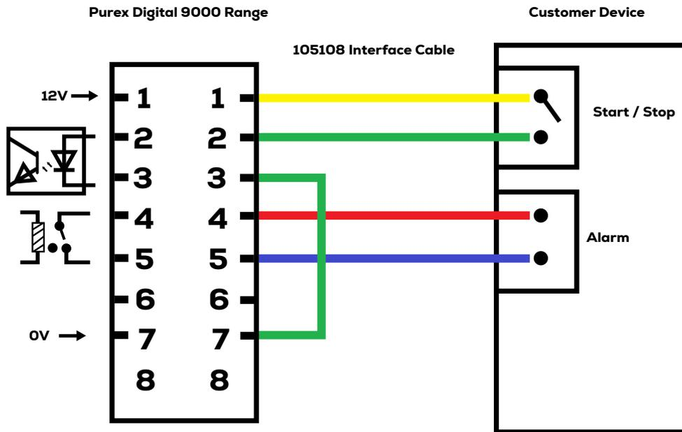
Using a 105238 cable the machine can be controlled remotely with a 9-24V signal. Below is an example connection to a host machine.
