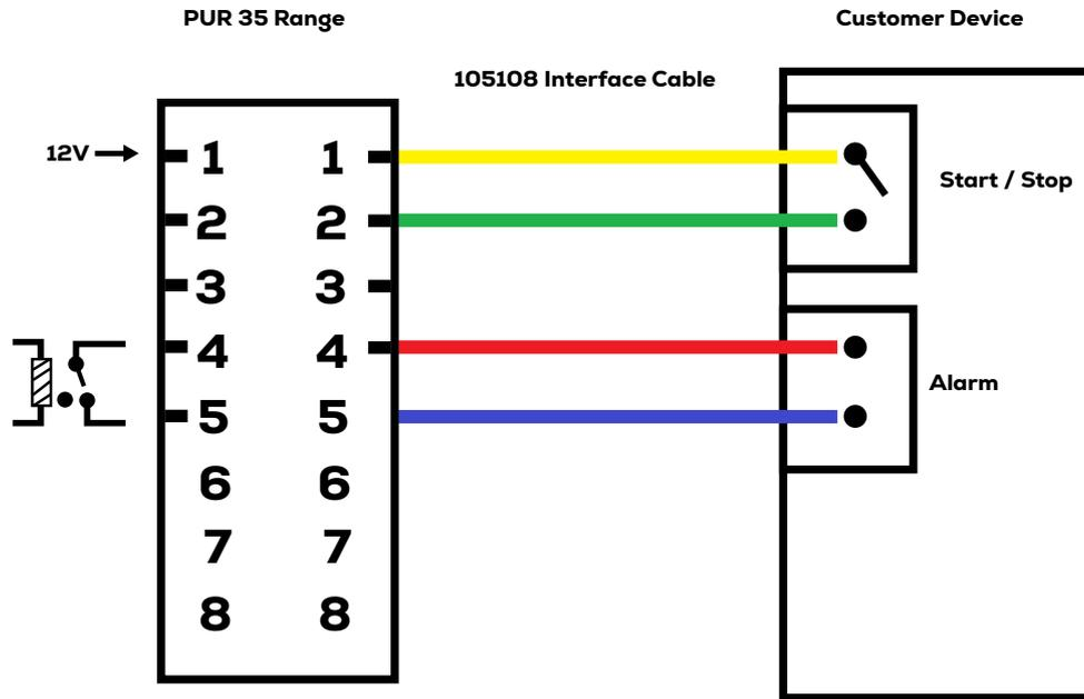
Using a 105238 cable the machine can be controlled remotely with a 12V signal. Below is an example connection to a host machine.
